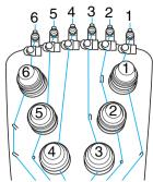
Pass the thread through the number 1 hole in the thread guide just above the spool, and then pass the thread through the number 1 hole in the thread guide toward the front of the machine.
